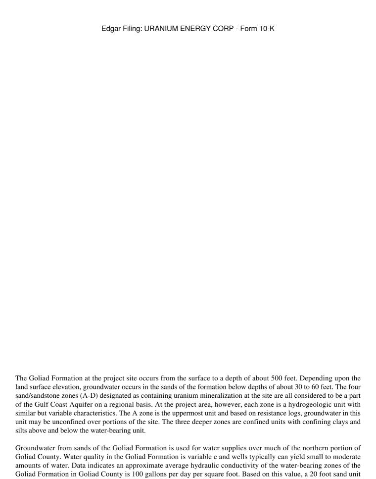
would have an approximate transmissivity of 2,000 gallons per day. With sufficient available drawdown properly completed ISR wells could have average yields in the range of 25 to 50 gallons per minute.
